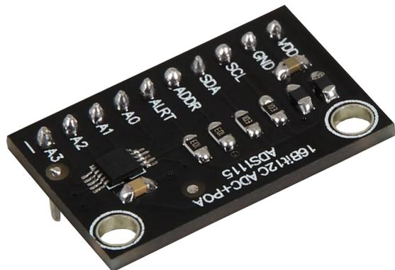
The pins A0 - A3 of the ADC are the 4 analog input channels. Thus, 4 analog sensors can be operated simultaneously.
