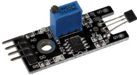
For the use of the magnetic sensor you additionally need the ADC.
